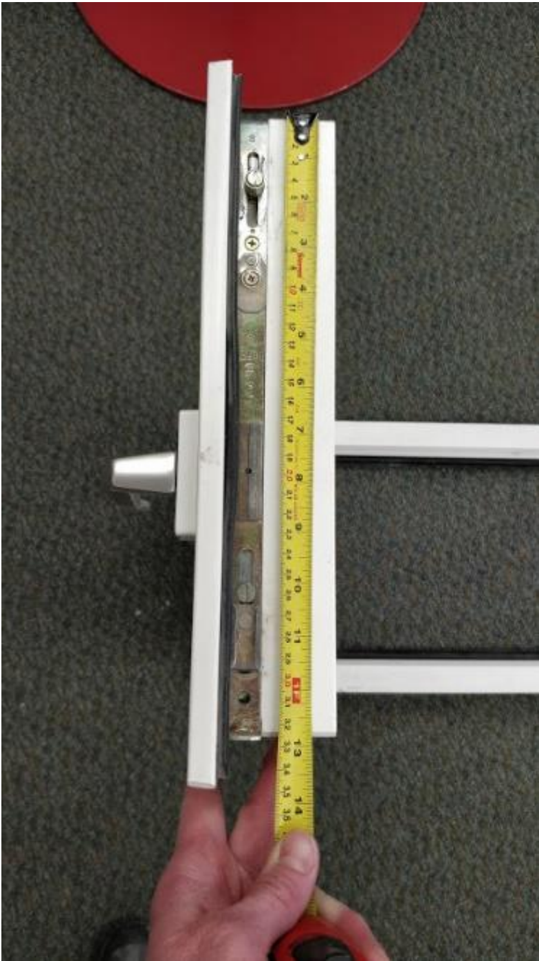
Measuring the hardware track. This track measures 12 13/16" (or 325mm).
