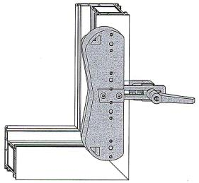
Inserting to frame rebate edge
