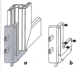
Inserting in fitting groove (a) Adjusting to groove width (b)
